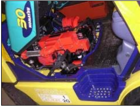
A standard forklift converted into an EX truck by Pyroban.
