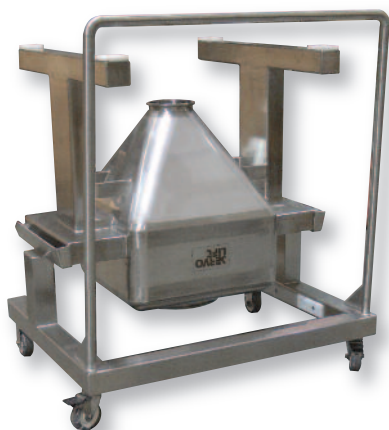
ERGONOMIC CARTS TO AID HANDLING LAB SIZE IBCs
